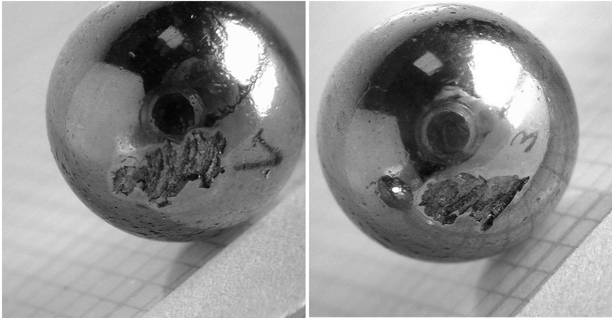
Figure 3: defective balls of the NDE bearing (among a total of five defective balls)
