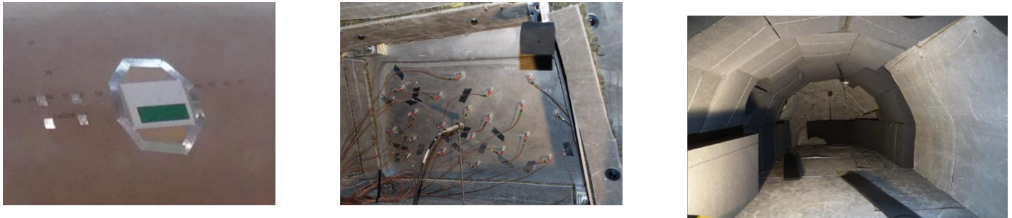
Figure 5 : View of the instrumented Mock-up / Wall pressure surface array (left), instrumented vibration panels (middle) and interior noise cavity (right)
